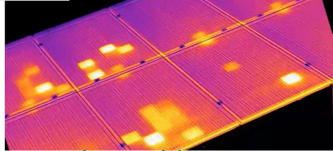
Inspecting solar panels enable
