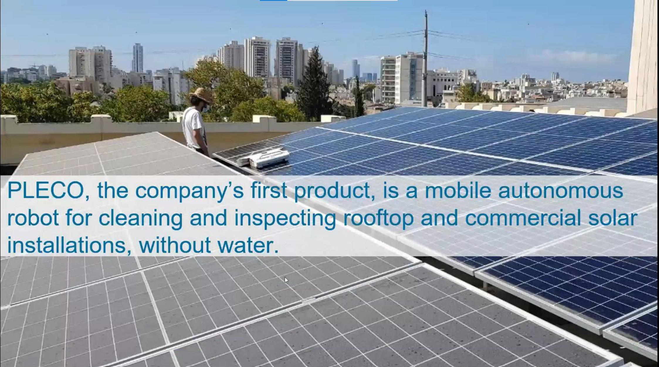
PLECO, the company's first product, is a mobile autonomous robot for cleaning and inspecting rooftop and commercial solar installations, without water.
